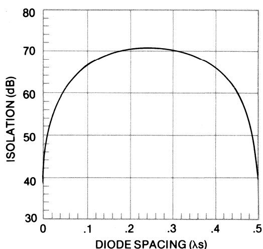
FIGURE 10.10-6 TWO SHUNT-ITERATED MA-4P404 DIODES — ISOLATION VS SPACING
