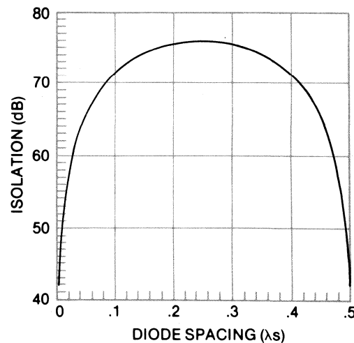
FIGURE 10.12-6 TWO SHUNT-ITERATED MA-4P505 DIODES — ISOLATION VS SPACING
